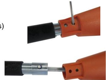
The 2 boreholes for the push button at the drive shaft serve as length adjustment between shaft core and protective hose. **The shaft core should be freely movable in length and must not get compressed.**
