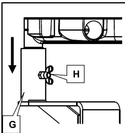
The cutting system is connected to the feed unit via the front guide roller.
