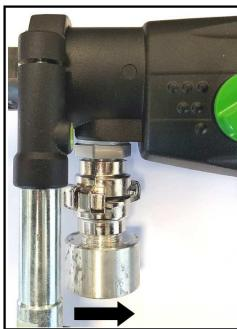
Dust which occurs during your work is hazardous to health. That is why it is advisable to use a deduster and to wear a dust mask on dry drilling. Place the adapter for the dedusting unit onto the tool's connector and turn into the direction of the arrow up to the stop. As a suitable wet/dry deduster, our DSS 35 M iP is available as add-on. The use of a dedusting system is also a prerequisite for optimal cutting performance of the bit (air cooling).
