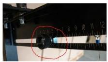
stopper screw for cutting depth
