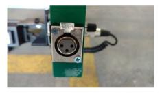
connector on bow for foot switch
