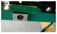
connector on bow for power supply
