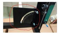
base plate for bow with 0 - 75 °-scale, top base plate for bow with 0 - 75 °-scale, bottom machine screw M6 x 45 mm metal washer, big self-retaining nut
