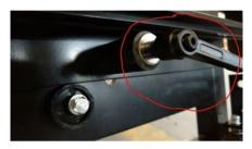
clamping device for °-adjustment of the support arm
