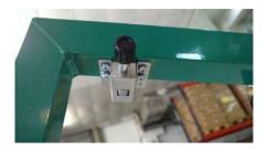
transport restraint, top transport restraint, bottom
