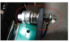
guide roller for hot wire allen screw M6 x 40 mm self-retaining nut M6 nut M6 cable shoe for power connection metal washer, small
