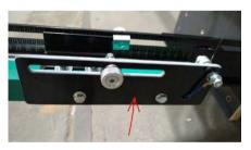
holder for hot wire tensioner, bottom, plastic machine screw M6 x 20 mm metal washer, small
