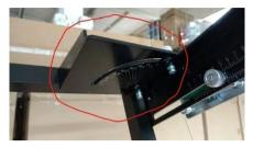
base plate for bow with 0 - 75 °-scale, top base plate for bow with 0 - 75 °-scale, bottom with reinforced sides machine screw M6 x 45 mm metal washern, big self-retaining nut
