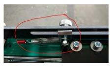
tension spring for hot wire, bottom knurled screw, metal M6 x 40 mm slot nut self-retaining nut M6
