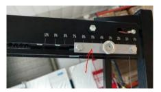
support plate for adjuster for slanted cuts knurled screw, metal M6 X 25 mm slot nut M6 metal washer, small
