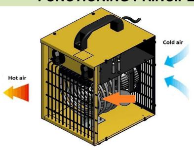
The device works on the principle offorced convection . The air flow is forced fan. Cold air is drawn in the back of the unit. Further washes flowing from the heater receives heat. The heated air is expelled in front of the heater. The device has a thermostat for the regulation temperatures 5-35  $^{\circ}$ C. The unit area equipped with thermal protection is acting automatically. The unit features: ventilation, heating with half the power, heating at full power.
