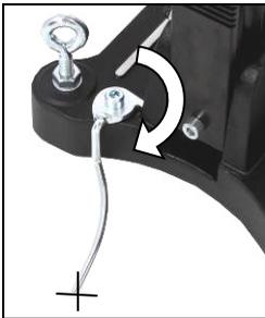
Mark the center of the hole to be drilled.
