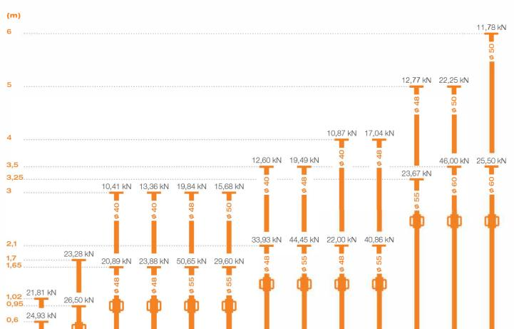
Testet i forhold til/ tested according to: UNE-EN 1065:1999 - Apart. 10.2
