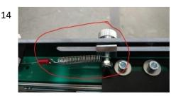
hot wire fastener (top) and adjuster for slanted cuts machine screw M6 x 40 mm tension spring for hot wire, top guide roller for hot wire self-retaining nut
