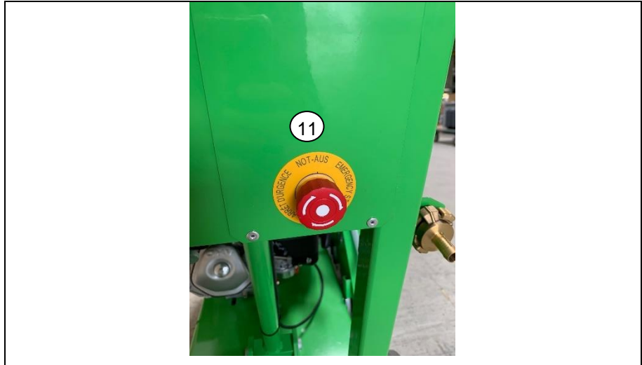
Abbildung 6: emergency stop switch
