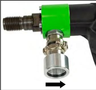
Dust which occurs during your work is hazardous to health. That is why it is advisable to use a deduster (Dust class M) and to wear a dust mask on dry drilling. Place the adapter for the dedusting unit onto the tool's connector and turn into the direction of the arrow up to the stop. As a suitable wet/dry deduster, our DSS 35 M iP is available as add-on. The use of a dedusting system is also a prerequisite for optimal cutting performance of the bit (air cooling).
