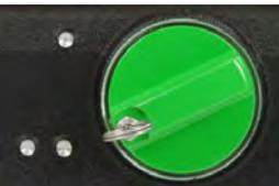
The **ESD 200** is equipped with a mechanical 2-speed oil-bath gearbox. Select the speed according to the drilling diameter (ref. to the tool's identification plate). Loosen the detent bolt on the gear change switch and turn the gear change switch as far as it will go into the faster or slower gear.
