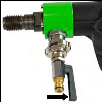
Place the adapter with the ball valve onto the tool's connector and turn into the direction of the arrow up to the stop. Connect the tool to the water supply system or a water pressure vessel using the push fit nipple.
