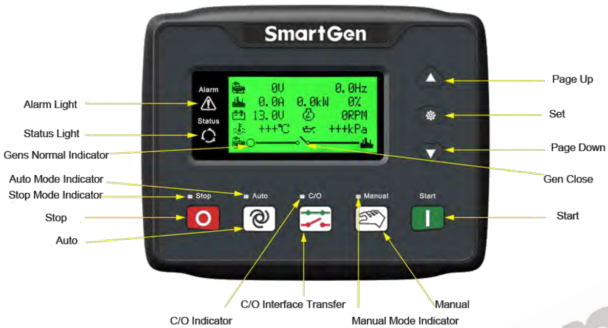
Fig.1 - HGM4010N/HGM4010NC/HGM4010CAN Front Panel Indication
