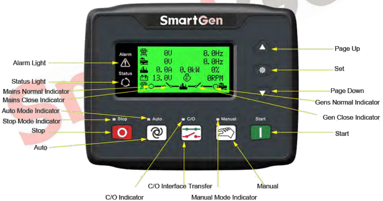
Fig.2 - HGM4020N/HGM4020NC/HGM4020CAN Front Panel Indication
