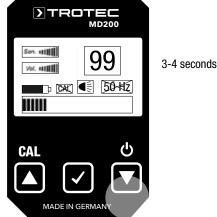
Pressing the "Down key" for approx. 3-4 seconds switches the device off.
