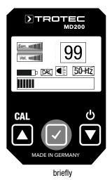
Actuation of the "confirmation key" activates the selected submenu. It will be displayed in black inverted.
