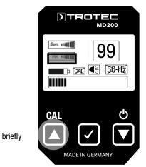
If the menu item "sensitivity" is activated (Sen black inverted), you can adjust the sensitivity by briefly pressing the Up or Down key.
