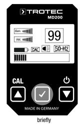
If the menu item "illumination" is activated, you can switch the illumination on or off by briefly pressing the "confirmation key".
