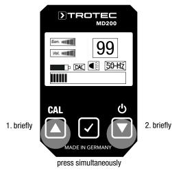
If no submenu is selected, the display can be rotated by 180° by means of simultaneous actuation of the "Up" and "Down" keys.
